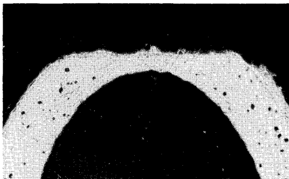
Fig. 13 Erosion of chamber tube. a) Cross-sectional view of a main chamber. b) Portion bounded by circle A, normal tube. c) Portion bounded by circle B, eroded tube.
